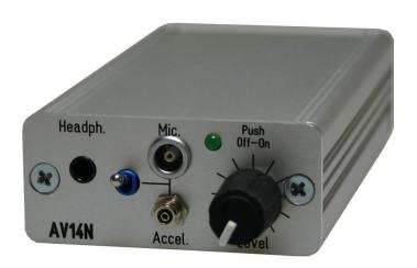
The 1-channel charge amplifier AV14 is a small battery-driven instrument, which has been constructed mainly to monitor acoustic and vibration signals. It has a measuring channel for an electret condenser microphone or a piezoelectric accelerometer. The switching over from the accelerometer to the microphone comes automatically, when the microphone mini-jack is plugged in. A headphone output is built in for monitoring purposes. The loudness of
